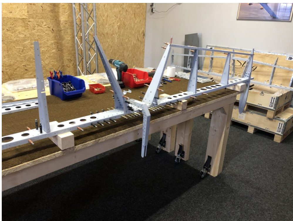
The balance counter weight holes in elevator rib 4 need to be enlarged to fit the big 4.8mm rivets.
