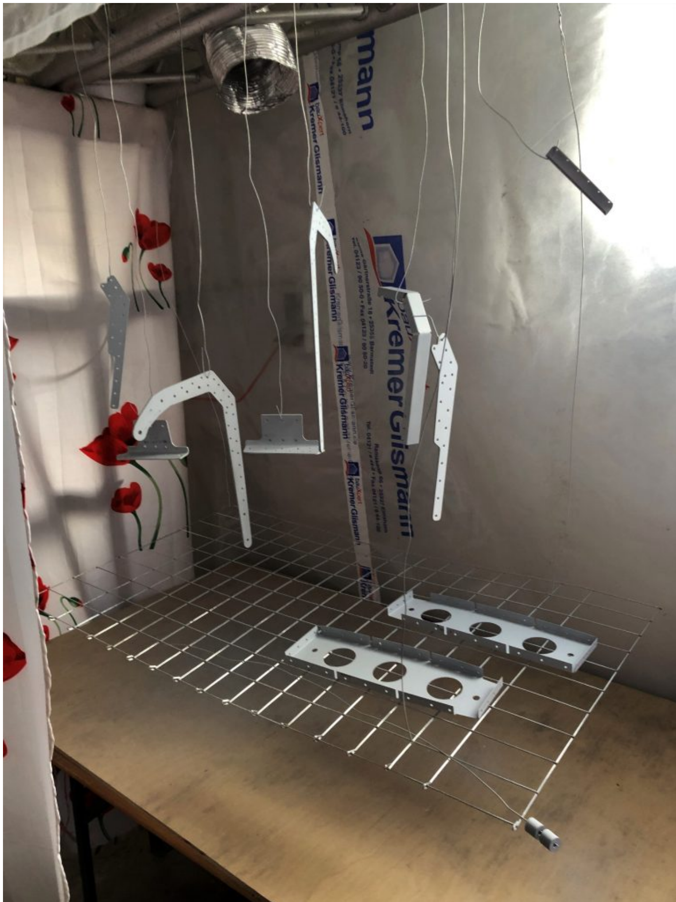
Paint booth with exhaust fan mounted to a flex pipe. The nice flowers are from grandmas never used shower curtain.
